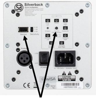
RAM TWEAKS are installed through the USB on the Silverback module and by pressing the Connect button
