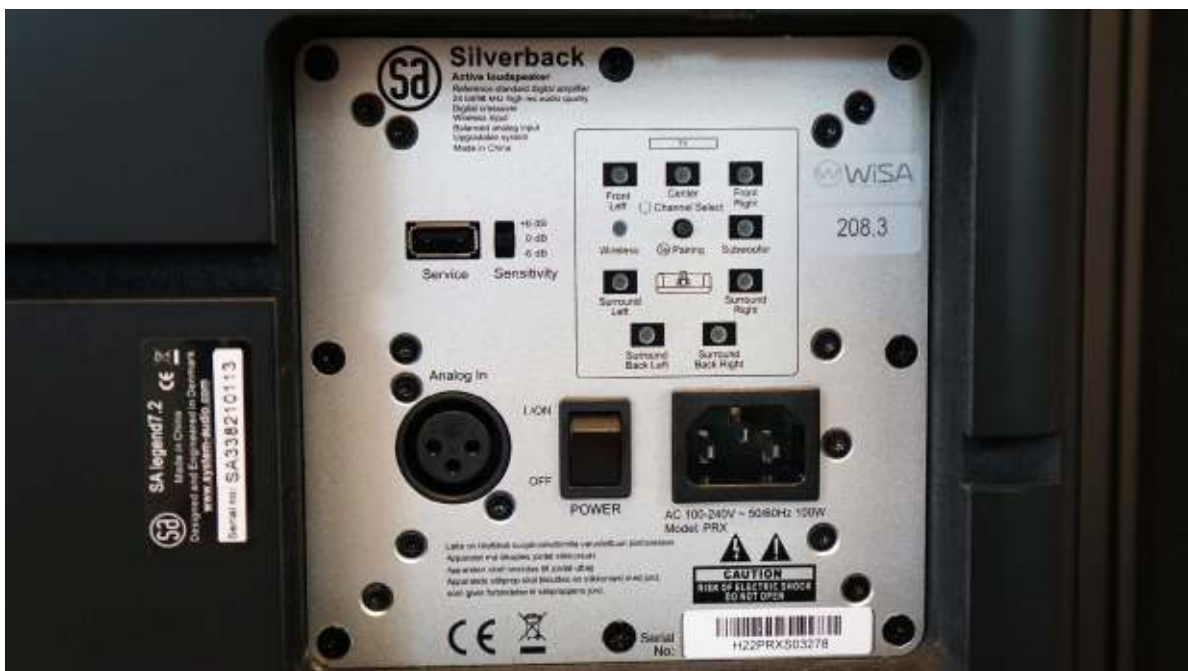
SA Legend's rear panel controls includes a balanced analogue input and power. The speaker's position is selected from eight options (boxed out section) using the central pairing button. There are also three sensitivity settings for -6dB/0dB/+6dB
